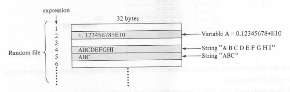
All numeric variables, including those represented exponentially, are 32 bytes or less long. However, a string has a maximum length of 255 bytes and one whose length exceeds 32 bytes cannot be stored in a single record of a random file.
