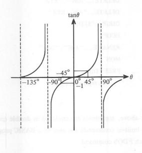
In this sample program, "OVERFLOW" is displayed when overflow occurs upon calculation of the tangent on line number 120. Actually, when TH=90, TAN  $(\pi/2) \rightarrow \infty$  and overflow results. Control is then transferred to the statement on line number 1000, "OVERFLOW" is displayed and the statement on line number 1010 returns control to the main program.
