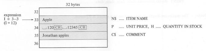
A sample program which reads the random file generated in the above manner is shown below. Variables to which the values stored in the same record are assigned are separated with a semicolon in the INPUT # statement. If the value for P is stored but no value for H, 0 is assigned to H. That is, if no corresponding data is sotred, numeric variables are set to 0.
