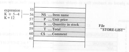
As shown in the above example, data can be stored in any specified records; therefore, empty records can be generated in the random file.
