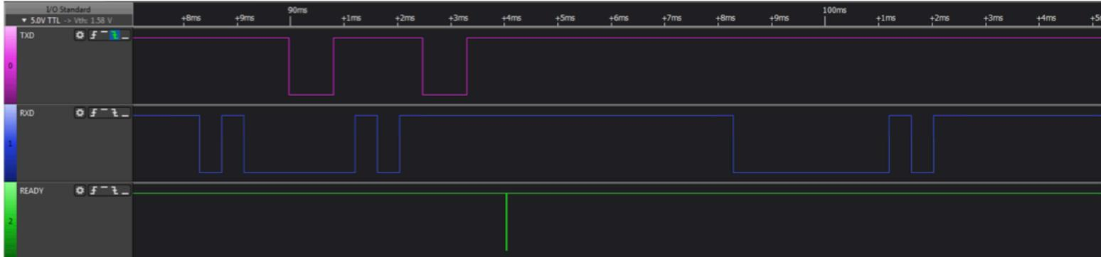
Up close, the keyboard transmitting key 'A' press (scancode 0x1E) to the host.
