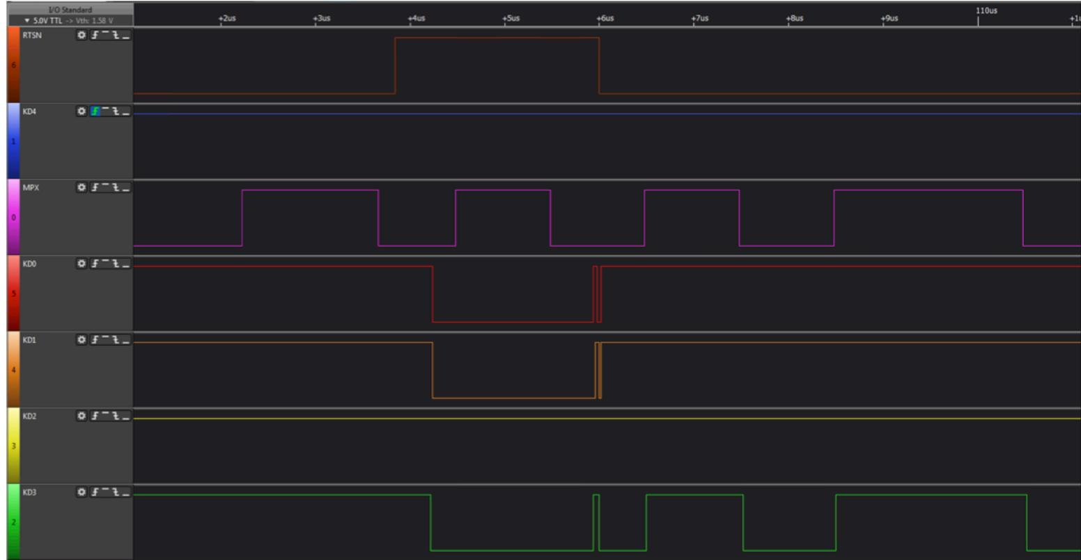
The timing delay between RTSN going active and row data being available can be seen in this diagram. Unfortunately I seem to have mislaid the timing diagram showing KD4 trailing RTSN, next time I rig up the logic analyser I will snapshot it.
