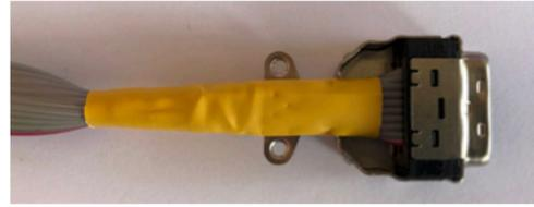
The ribbon cable and plug are then placed into the metal case and secured with the cable clamp screws. The case lid is placed on top followed by the hood.
