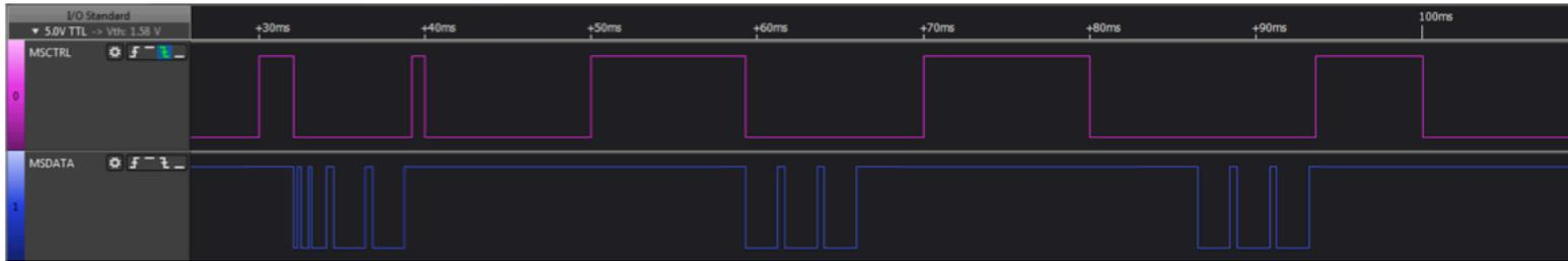
The mouse is stationary with the Left Key pressed.
