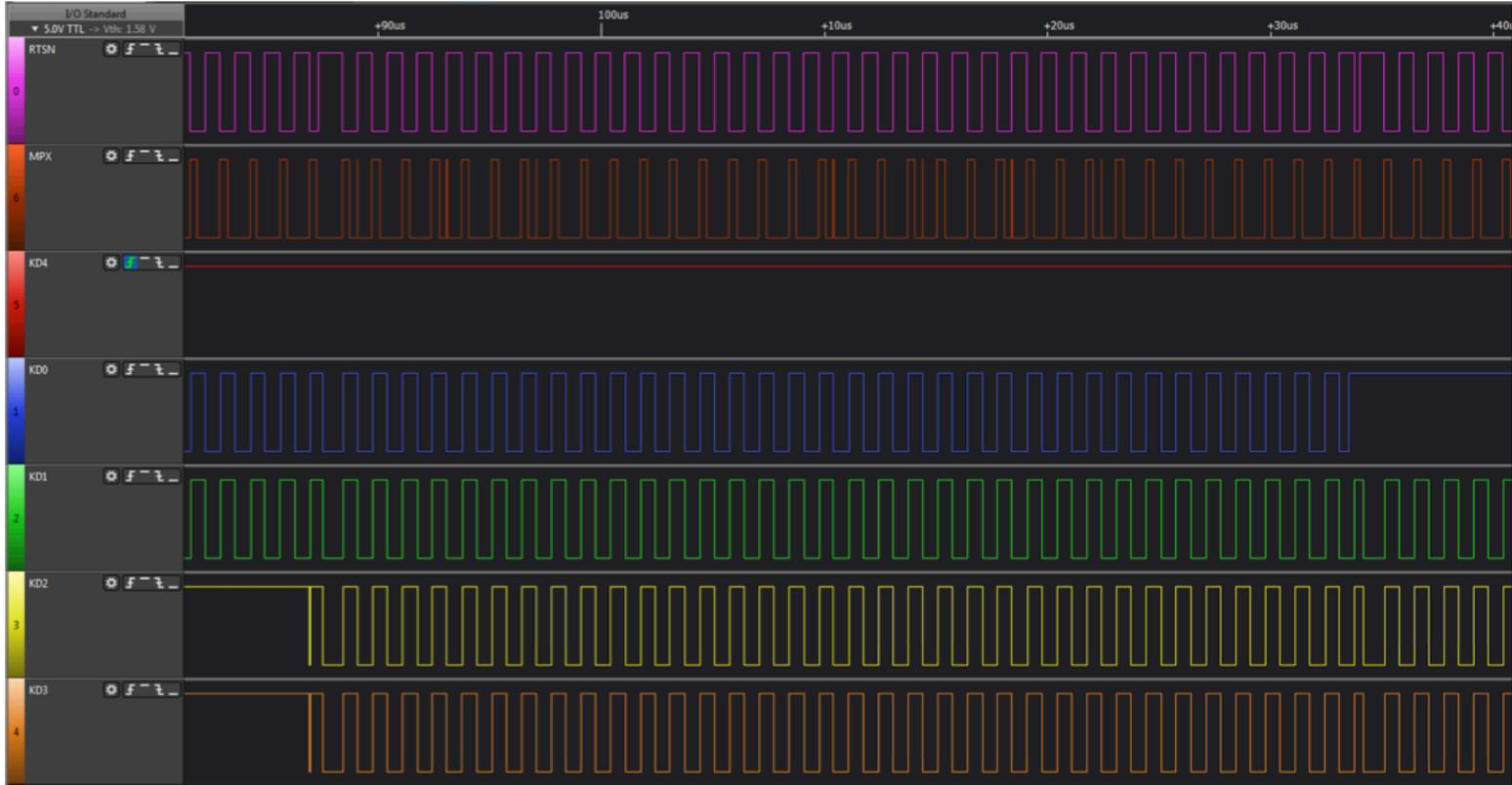
Once row 11 and 12 have been probed, the mainboard commences a sequential scan of all the rows, starting at row 0, looking for the pressed key. Again look at the wide RTSN signal pulse and you will notice KD[3:0] incrementing.
