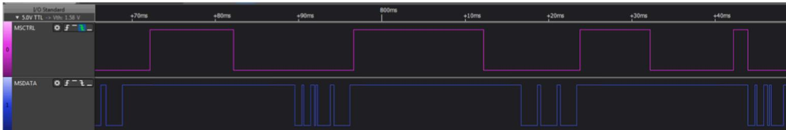
The mouse is stationary with the Middle Key pressed.
