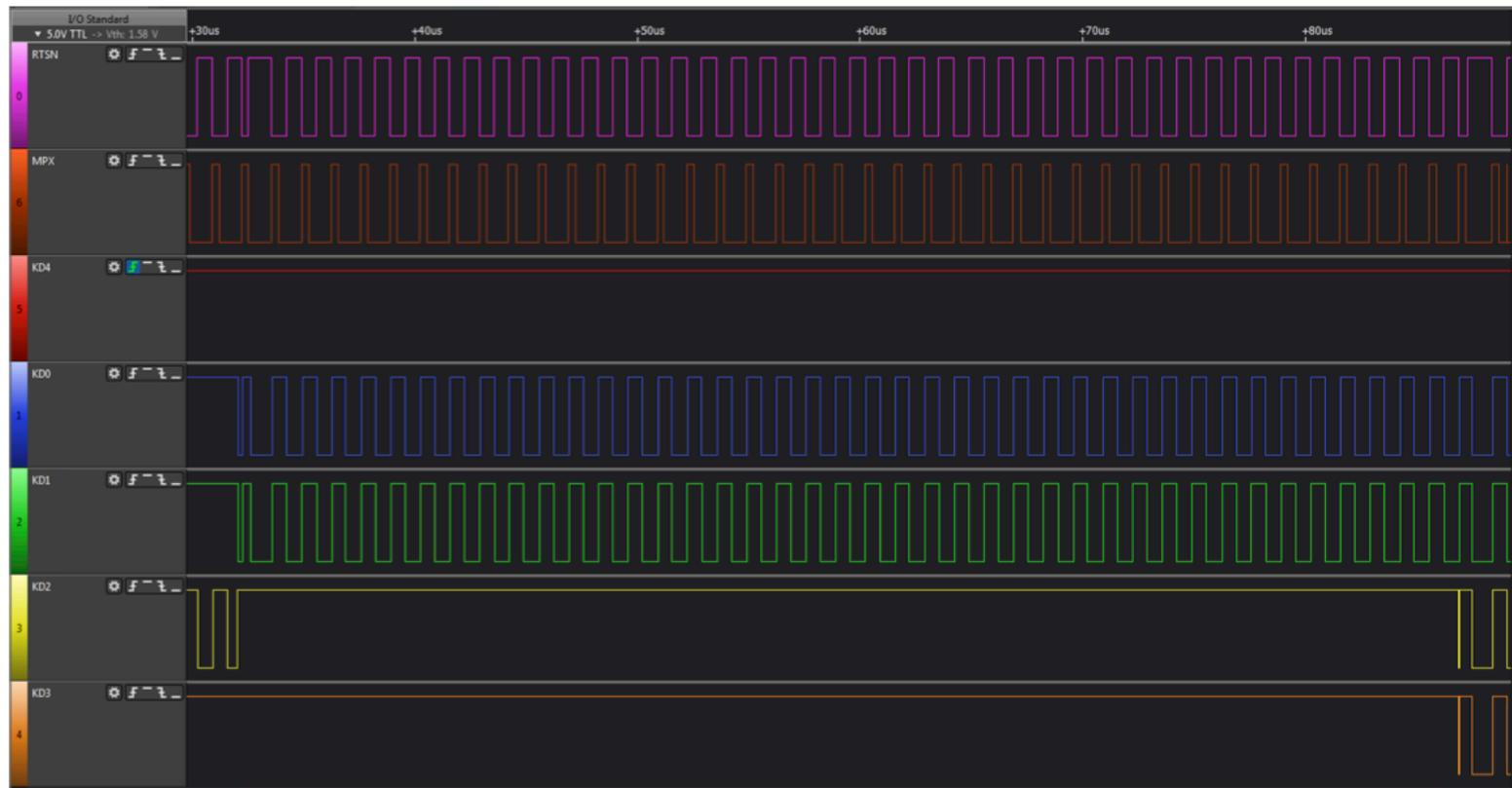
After probe of Row 11 it switches to Row 12 which contains the Japanese Transform keys. This can be seen on the left of the image, the wide RTSN pulse, look at the KD[3:0] values below and it will read 12 in binary. Row 12 is then scanned for around 50us.
