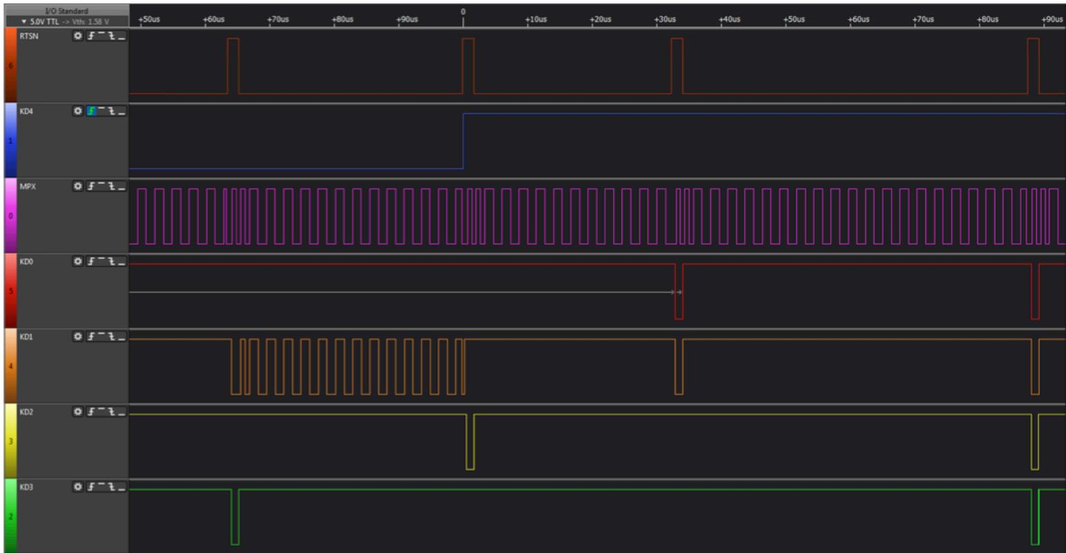
Once a key has been pressed, the mode changes to key retrieval mode. KD4 goes HIGH and the mainboard starts sending valid row numbers to retrieve column data. As per the MZ-2500, row 11 is interrogated first followed by row 12 and then a sequential sweep from row 0 occurs.
