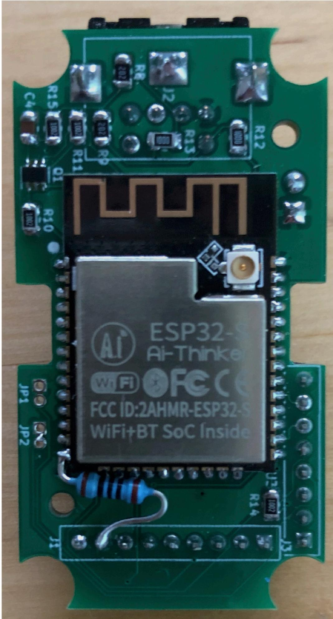
Modification required to an mz25key to allow it to run SharpKey firmware. A 100R resistor is placed between pin14 (GPIO12) of the ESP32 and pin 8 of the host interface header J1.
