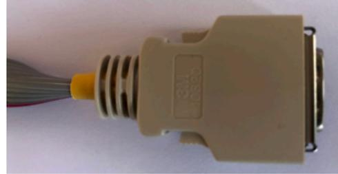
The unconnected end of the ribbon cable is then wired according to the diagram below, the red identifier cable is Pin 1, ie. 5V.
