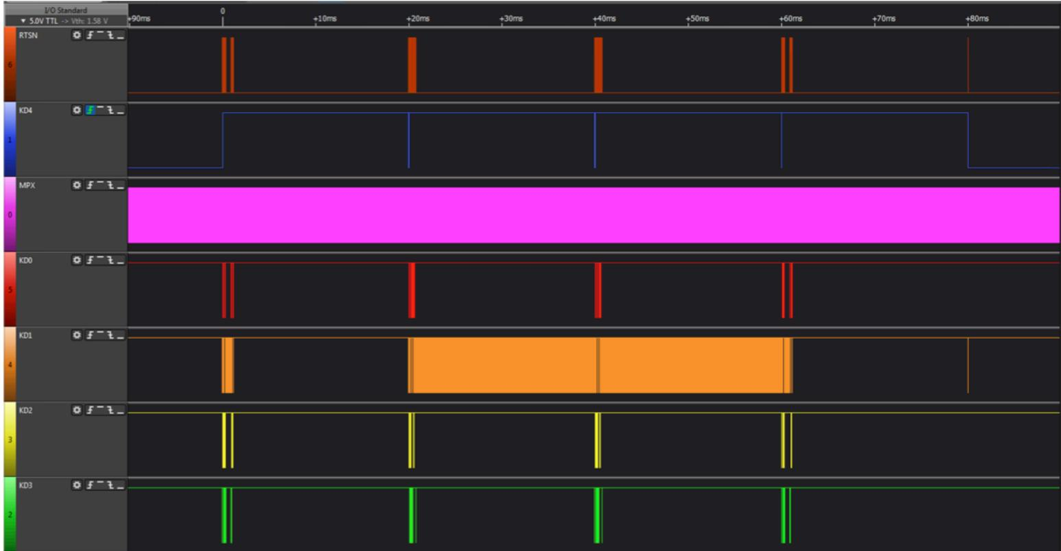
A full cycle, where a key press is detected until the moment it is released.
